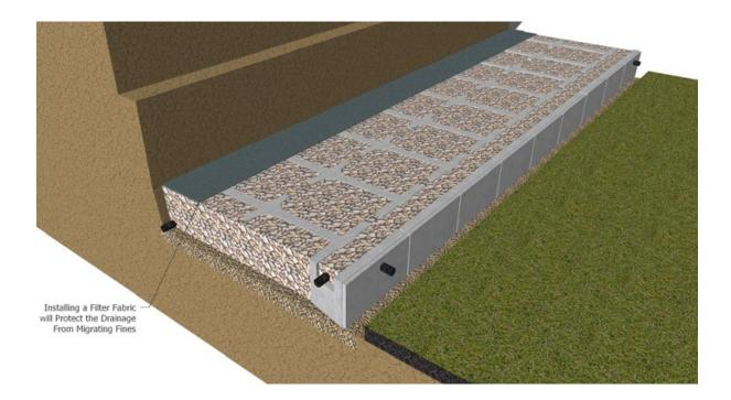
Install a soil separating fabric (Filter Fabrics) to separate the fines and compacted backfill material from the drainage aggregate. The filter fabric can be installed directly behind the MagnumStone® extender units. They can also be installed directly on top of the drainage gravel.
