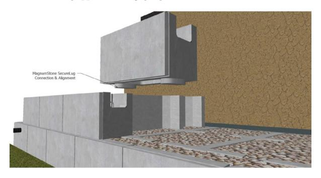
▶ Lay the next row on a running Bond pattern with the SecureLugs connected in the hollow core below. The SecureLug Connection provides a strong block to block connection and alignment throughout building your retaining wall.
