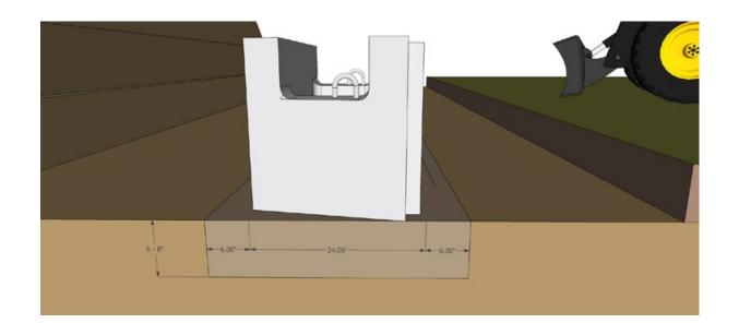
The Leveling Pad Trench Depth should be cut out to approximately 6" (150mm) from the back and the front of the total depth of the base course. For instance, MagnumStone® Standard Unit 24" + 6"(front) + 6"(back) = 36" total (610mm + 150mm + 150mm = 910mm).
