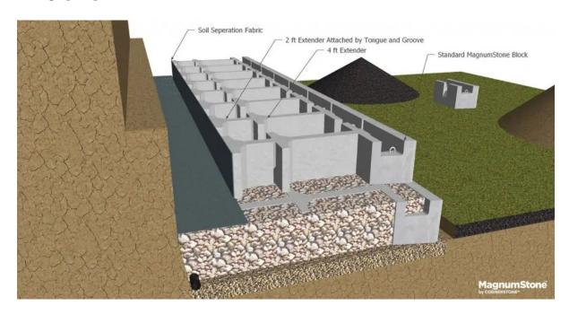
■ Continue to place the MagnumStone blocks on top of the retaining wall blocks below. Ensure they are level front to back ans side to side. Small adjustments may need to be made during the construction process. Soil separation fabrics can be added wherever the backfill meets the drainage gravel to keep fines from migrating into the drainage zone.
