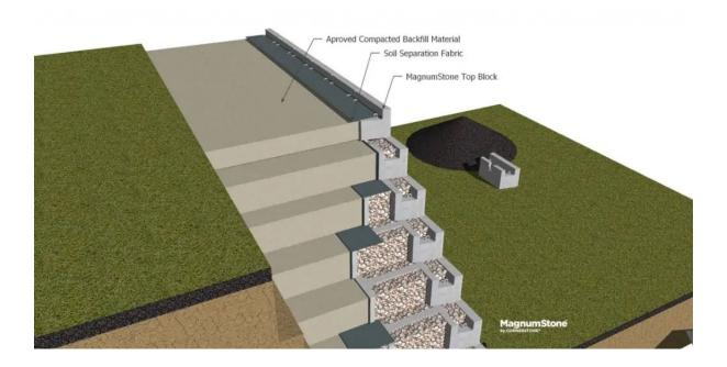
Install the top MagnumStone retaining wall block like the rest of the wall. The top block will not have the back edge on the top. This is the location that the soil separation fabric will lay to protect the hollow core and drainage channel of the block.
