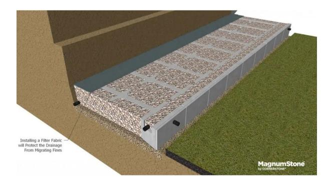
Install a soil separating fabric (Filter Fabrics) to separate the fines and compacted backfill material from the drainage aggregate. The filter fabric can be installed directly behind the MagnumStone extender units. They can also be installed directly on top of the drainage gravels.
