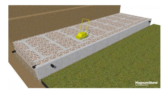
▶ Backfill the MagnumStone blocks and extender units with a clear crush gravel (#57 Stone) or equivalent slightly above the units. Run a plate vibratory compactor over the stones and units allowing them to settle in the hollow cores. Sweep any excess stones off the top of the units and blocks.
