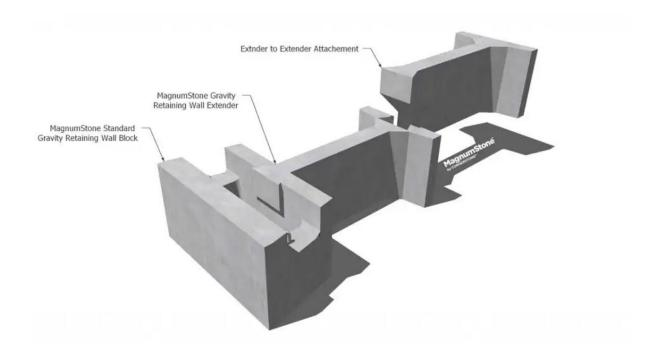
Place the tongue of the extender block inside the groove of the MagnumStone Base Block If extender to extender blocks are required place them in the same manner as the previous ensuring that the blocks stay level and true.
