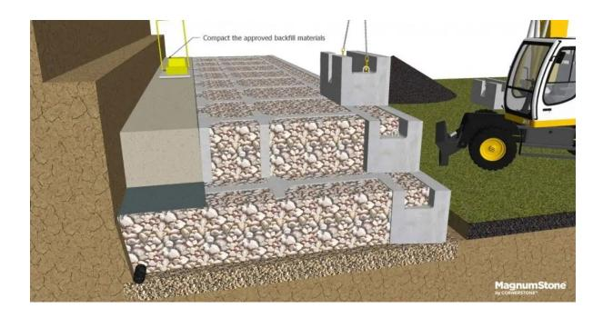
Compact the approved backfill materials in between the excavation cut zone and the back of the retaining wall blocks. Ensure that it compacted in lifts of no more than 8" and also compacted to 95% standard proctor density. It is crucial that these areas do not have loose fill where settlement can occur. drainage gravel to keep fines from migrating into the drainage zone.
