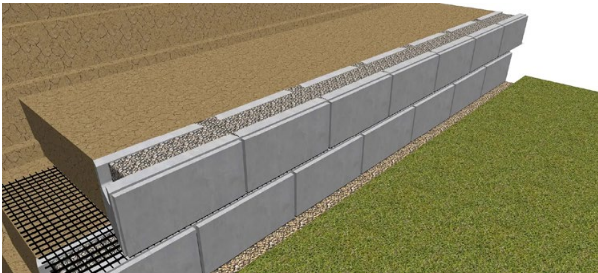
Second Row Drainage Gravel Installation for Retaining Wall
