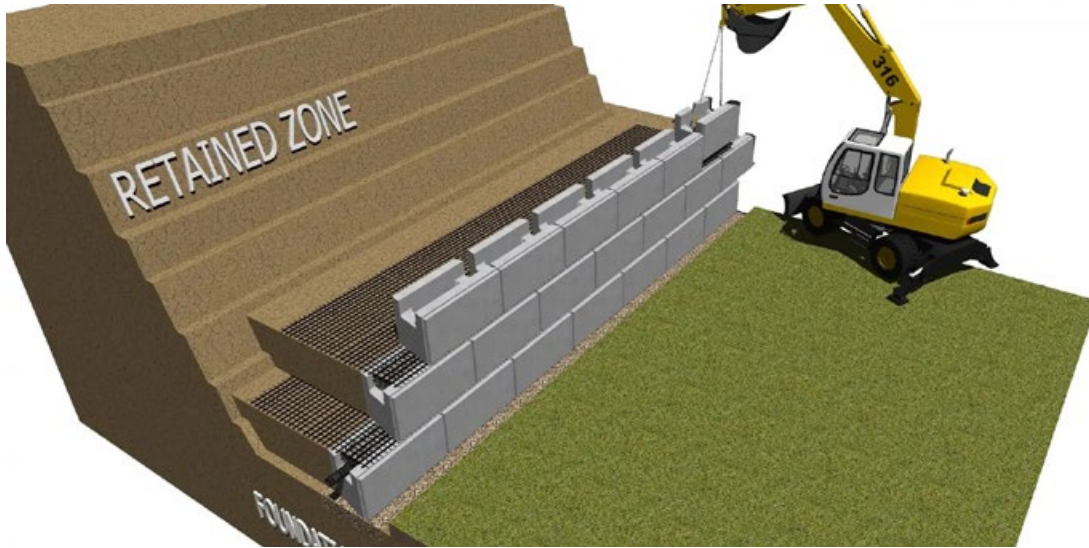
Installing 3rd Row of MagnumStone retaining Wall Blocks
