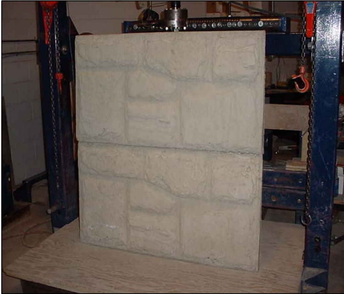
Figure 3: Photograph of the MagnumStone blocks in the connection frame
